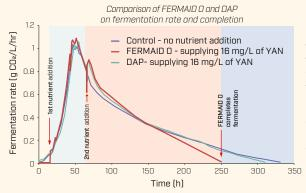
16 mg/L YAN was added at two stages of fermentation (at the beginning and at 1/3 of the alcoholic fermentation) in two forms: inorganic nitrogen (DAP) and organic nitrogen (FERMAID O™). This graph indicates the greater efficacy of FERMAID O compared to DAP on a per milligram nitrogen basis. Using FERMAID O results in a quicker finish to alcoholic fermentation.
